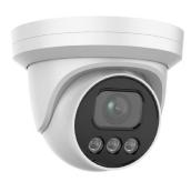
The Eagle Eye DT01 is a 4 Megapixel turret camera with an IP66 environmental rating. This model is suitable for indoor and outdoor use for a wide range of applications. The camera comes pre-configured to securely operate with the Eagle Eye Cloud VMS and Eagle Eye CameraManager.
