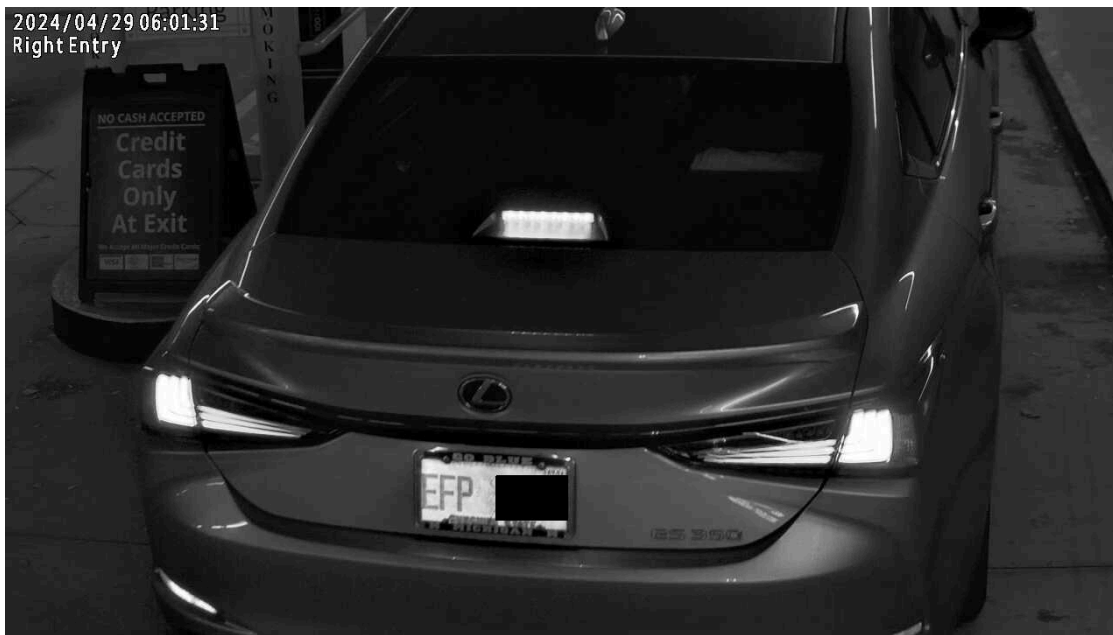
Figure 14: Both the license plate and vehicle make are visible in this IR mode image, due to sufficient light from an external source
