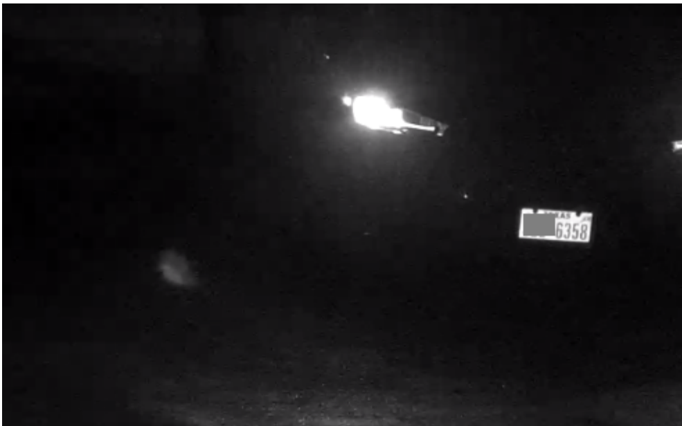
Figure 13: License plate capture at night under zero-lux environment
