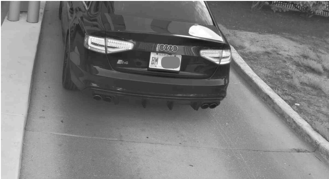
Figure 12: LPR detection using monochrome (IR mode) during daytime
