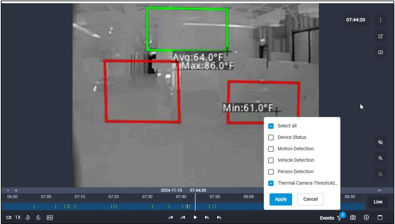
The display of bounding boxes and temperature is set up on the camera UI.
