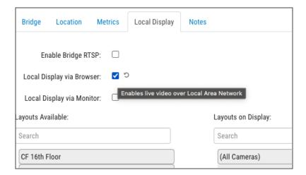
This option allows you to enter the IP address of the Bridge/CMVR WAN connection as a URL in your browser and to log in with your User ID and Password. This option will display the same layouts that are available for Local Display via Monitor in a browser window from a locally connected PC. This option is limited to displaying the Preview Streams from the local cameras, similar to Local Display via
