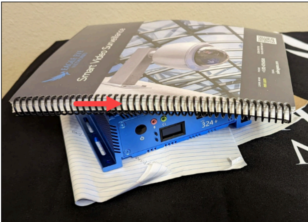
BAD EXAMPLE: DO NOT stack books or papers on top of the Bridge which can block ventilation and lead to overheating.
