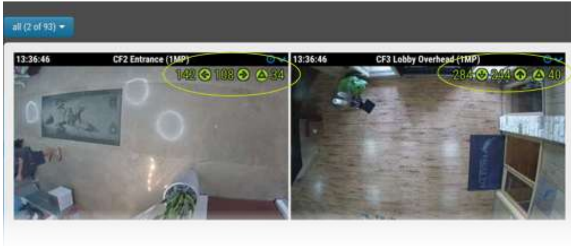
Image 4: Real-time tracking/counting of objects crossing a line in both directions including a total:
