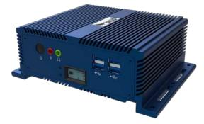
The Eagle Eye Bridge acts as a gateway from your premises to the Eagle Eye Cloud Data Center where your video is stored and managed by the Eagle Eye Cloud VMS. It provides a secure connection, video buffering, bandwidth management, and monitoring of cameras.
