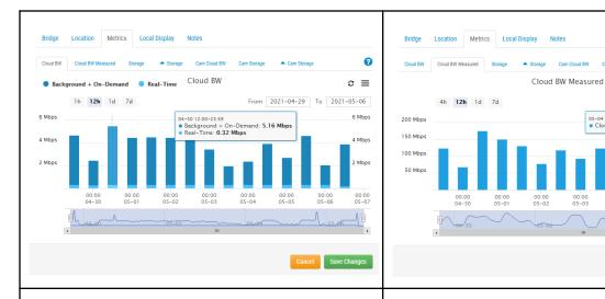
"Cloud BW" the synchronization of video to the cloud as well as the viewing of video that is not yet in the cloud. Real-Time is the preview video that is being transmitted directly to the cloud.
