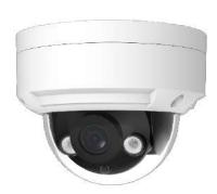
The Eagle Eye DD07 is a 4 Megapixel camera with an IP67 environmental and IK10 vandal rating. This model is suitable for indoor and outdoor use with a wide range of applications. The camera comes pre-configured to securely operate with the Eagle Eye Cloud VMS and Eagle Eye CameraManager.
