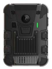
The Eagle Eye Body Camera BC01 is a cloud connected Body Camera. Extensive remote networking capabilities allow you to interact with the camera through 4G LTE and/or Wi-Fi networks. On-board capabilities include world-leading 180° immersive video capture at up to 4K resolution, bi-directional audio, GPS tracking, and high-performance Qualcomm<sup>™</sup> processing.
