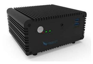
The Eagle Eye CMVR 225 and 325 family has a rugged, aluminum enclosure with integrated heat fins. It has 4 remotely managed PoE camera ports and is designed for demanding industrial applications. This fanless design makes no noise and has a wide operational temperature range. It directly supports 4 cameras on the integrated PoE ports and a total of 6 or 12 HD IP cameras with an additional ethernet switch.
