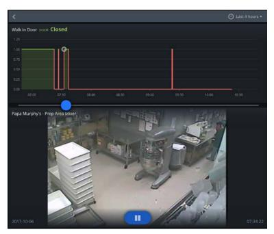
Because of the integration of Swift Sensors and Eagle Eye Networks cloud services, the Bertram's are now using Enhanced Video Notifications to obtain real-time video images anytime they receive a notification from the Swift Sensors network.
